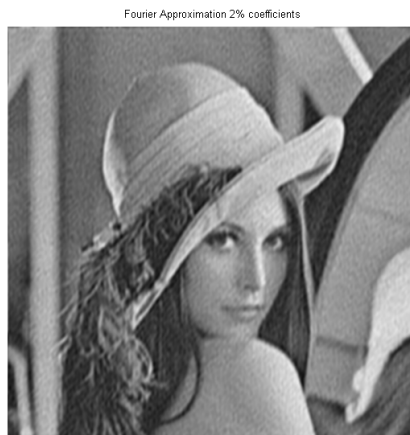
Fig. 4.27 Lena Image Fourier Approximation using only largest 2% coefficients
